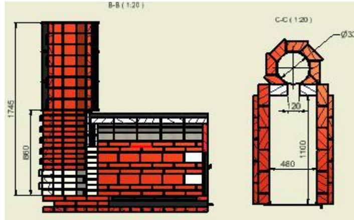
*Picture 2***Schematics of the heat transfer system.**
