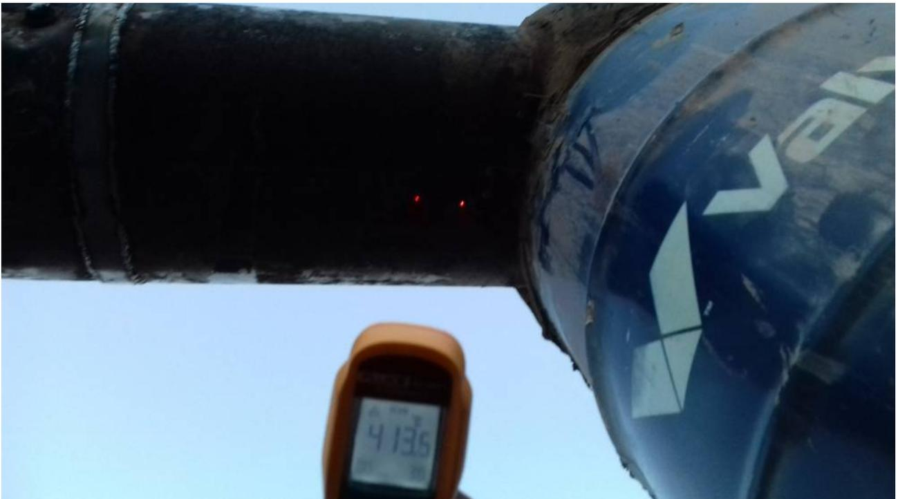
*Picture 26: Connection piece, next to the heat riser end. 19:22pm. Reading: 413,5 °C*
