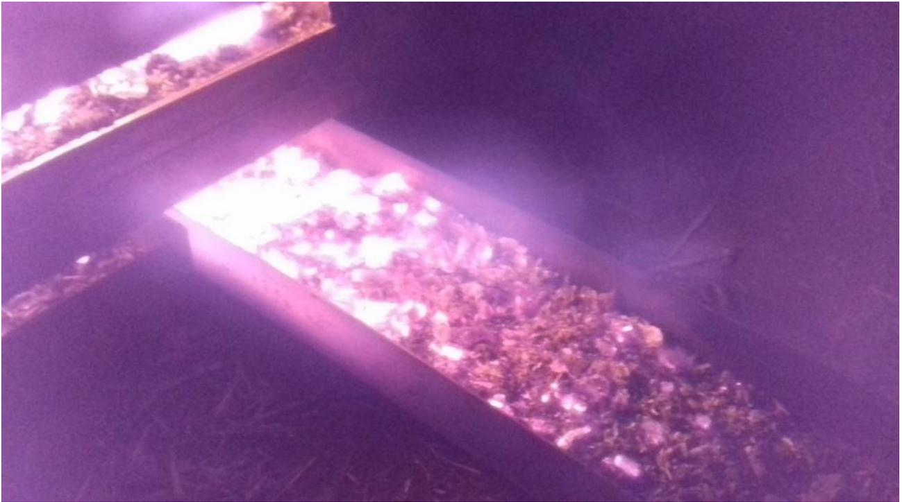
*Picture 18: 19:48 pm. One of the twin ash drawers. Part of the provisions to increase the burn rate is making space for the new wood. There was no floor isolation for this firebox, as the ash drawer with its cargo of ash (charcoal in this picture) provides the isolation for the wood burning above it. This metal drawer 2mm thick will have to be thickened to increase its life.*
