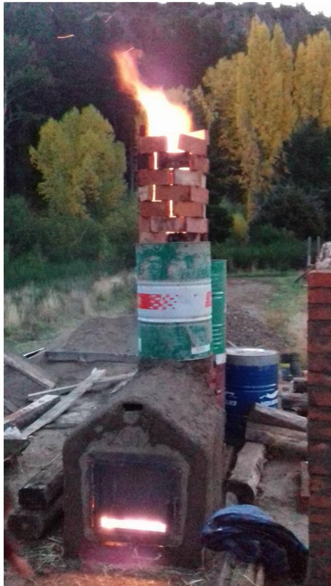
*Picture 17: The equivalent height of a 200l drum is added with bricks and the flames keep showing up. We agreed to add this height to the riser in the next day to preserve the metal parts from the flames*
