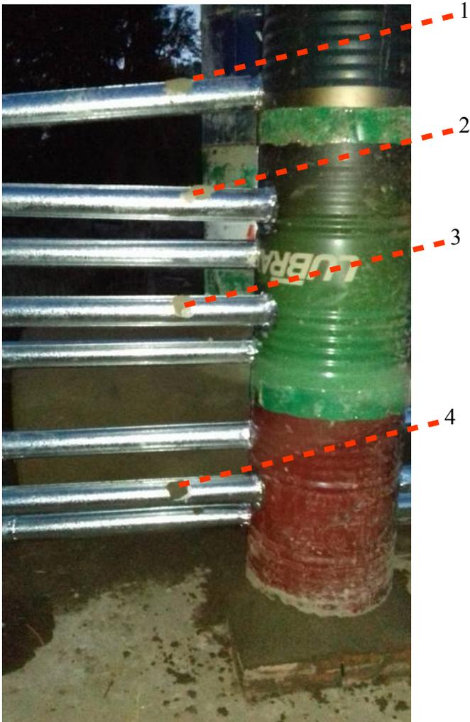
*Picture 21: 4 spots covered in mud to get a known emissivity (0,92) for the pirometer*
